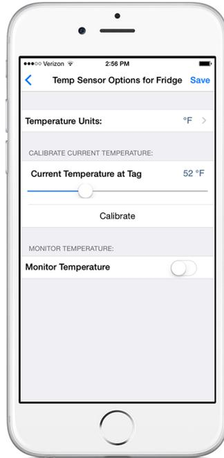
The temperature sensor often needs calibration to remove an offset. In the "Calibrate Temperature at Tag" section, set the correct current temperature, and tap the "Calibrate" button.
